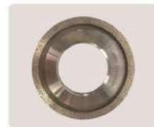
Golive four sides edger machine bottom grinding diamond wheel 150*76.2*10*5 140# For B type machine
