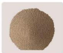
Silicon Carbide( for sanding machine) 24# 36# 60# 80#
