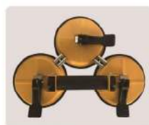
Suction Cup vertical capacity is 170kgs horizontal capacity is 200kgs dia 140mm thickness 8mm
